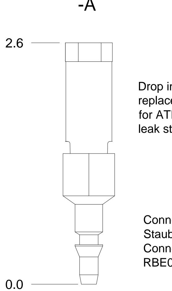
Drop in replacement for ATEQ leak standard
