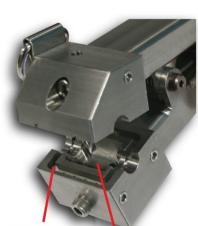
Outer chamber (Nitrogen curtain) Inner chamber (Helium measurement)
